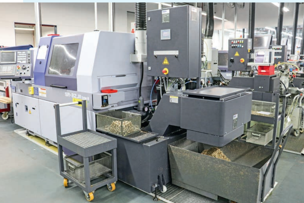
Connecting the LubiCool®-M device works according to the plug-and-play principle via six standardised hose couplings.
